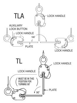
**HORIZONTAL LIFT:** Clamps (used in pairs or multiples) are attached to the side edges of a plate or bundle of plates positioned horizontally to the floor level. The rigging attached to clamps is generally multi-legged slings with the connecting point of the slings being approximately centered between the distance separating the clamps. Refer to illustrations shown below.
