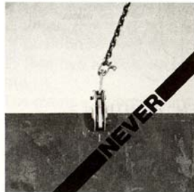
Photograph E (Typical) Excessive side-loading.
