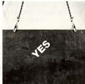
Photograph F (Typical) Clamps in line with sling.
